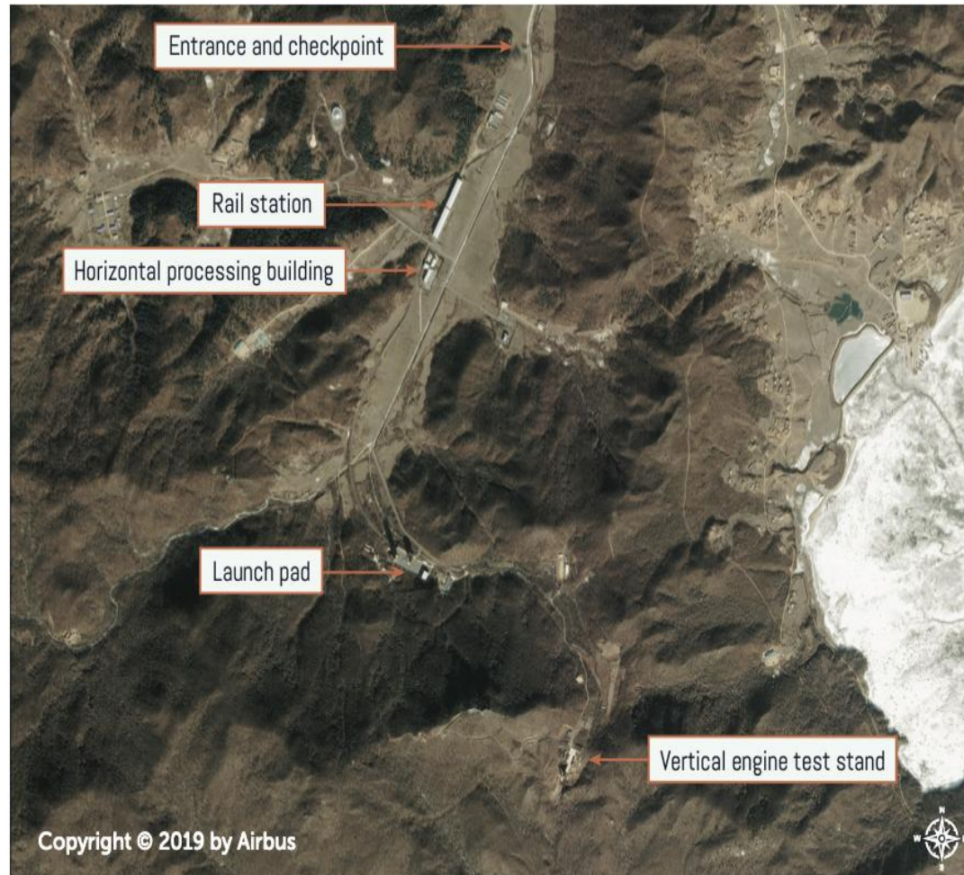
Satellite imagery of the Sohae Satellite Launching Station, January 20, 2019. Although disassembly appeared to be underway in July 2018, the vertical engine test stand (right) appears to have been untouched since August 2018. Photos: Airbus/CSIS Beyond Parallel
